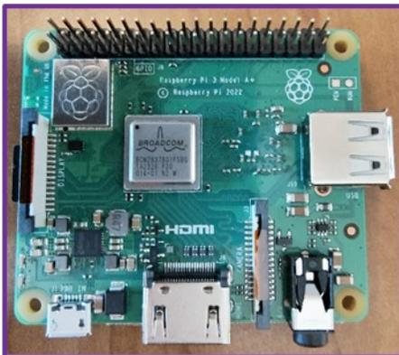
Here's what the Pi3 A+ looks like (left). You can see it's a bit smaller than the Pi3 B+, and some ports are omitted. Other than that, it connects to power with a microUSB connector (lower left), and the 40-pin connector header is devoted to the MMDVM board.
