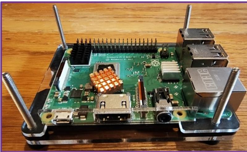
Here's a look at the Raspberry Pi 3 B+ board installed in an early step of the case assembly. You can see that the case pieces mate perfectly with the micro-USB, HDMI, and audio connectors on the front. The board fits snugly inside the case pieces and doesn't move around at all.
