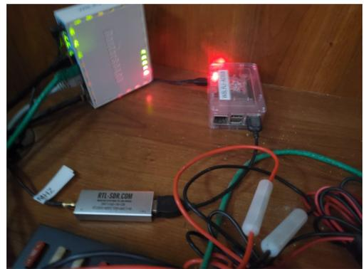
Before firing up the RPi, connect everything together as shown in the photos. The antenna is connected to the 1090 MHz bandpass filter which then goes to the LNA4ALL low-noise amplifier. This is connected to the RTL-SDR via an SMA connector and then to the RPi over a USB cable.
