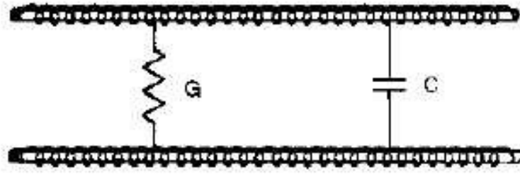
A. SHORT SECTION OF TWO - WIRE LINE
